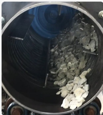
07. Dust removal equipment for Limestone
